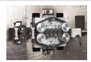
Powerful Servo Driven Drive System – for processing of the most demanding applications. Separate closed-loop encoder independently measures wire and self corrects for any slippage, assuring accurate wire lengths.
